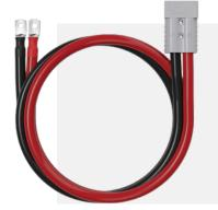
The **RING to Anderson Connector Adapter** is a 10M extension lead with 6 AWG high-purity, oxygen-free tinned copper wire for maximum conductivity. Designed to withstand temperatures from -40°C to 105°C, with silver-plated contacts for durability, this cable meets high standards and performs reliably under harsh vibration conditions. **RPC3306SR-50-SCA-G1-AU**
