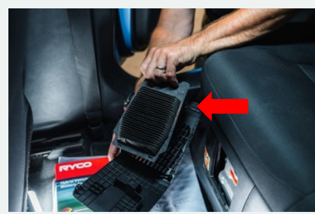
STEP 6 Repeat above steps in reverse to re-install OEM battery air filter housing flap.
