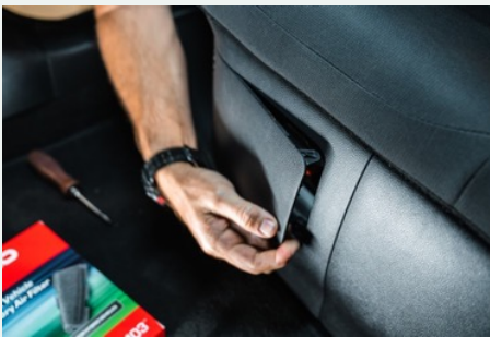
STEP 4B Using flat head screw driver or hands, wedge in-between around perimeter of battery filter OEM housing flap and back seat to begin removal of housing flap - then gently pull open flap to release remaining tabs.
