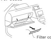
Open the glove box and remove the cover located at the back of the glove box. Do not remove glove box.
