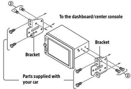
When mounting this unit to the preinstalled brackets of your car, use the supplied screws ② in the appropriate screw holes based on your car: T for TOYOTA and N for NISSAN.
